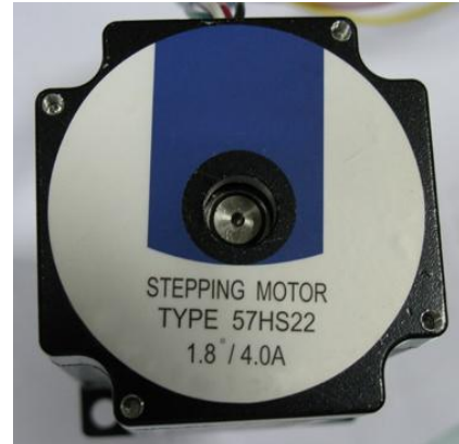
Motor nameplate/ stepper angle=1.8°
