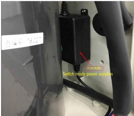
2.1) If output voltage of switching mode power supplies lower than DC18V, the life and flow of pump will affect due to low voltage, it can be judged as failure of switching mode power supplies or pump failure.
