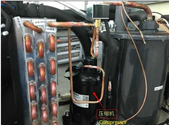
Observe whether the compressor is vibrating when the thermostat reaches refrigeration status (D2 of thermostats light on). If there is no vibration of the compressor and the surface of the compressor gets heating, it means the interior of the compressor has malfunctioned.
