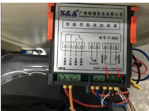
1.1) If the alarm stops can be judged as the terminals poor contact, and then reconnect the wires back
