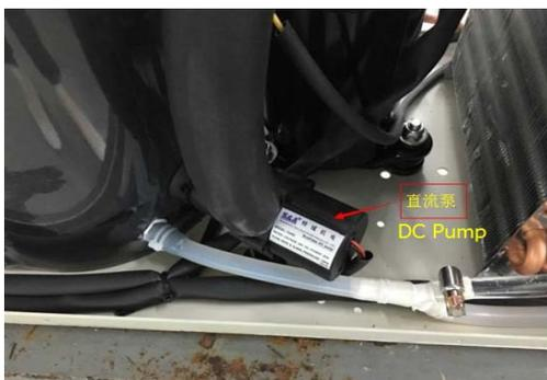
**Solution:** Take away the shell of DC pump and check if there is choking or wore in rotor. If the alarm continues, it will need to replace DC pump.
