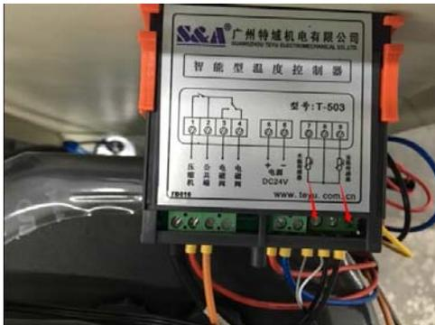
1.1) If the alarm stop can judge is the terminal poor contact, reconnect the wires back to original terminals.
