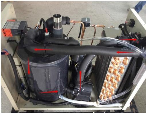
Clean the pipes to remove blockage or replace the bending or damage pipes.
