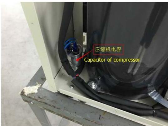
3.2) Check input voltage of compressor with testing tools (depending on the model: please refer to the manual technical parameters), if voltage lower than compressor boost voltage, the compressor do not work.
