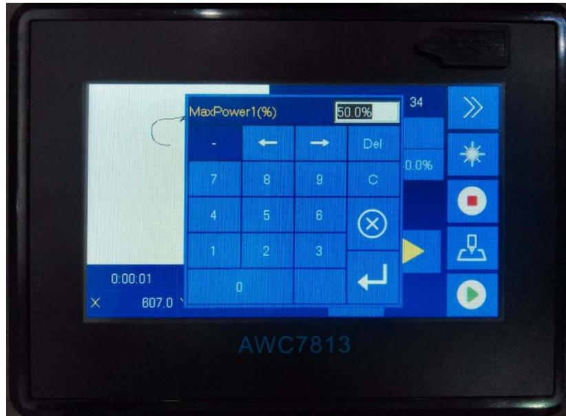
**Figure3-10-2-2 Modify the mini power of the file being processed**
