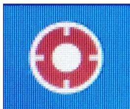
In the [Figure3-1-2 Main interface 2](#), after clicking the **【Reset】** button, the laser head will move in the X-, Y- direction. When it touches the X-, Y- limit switches, the laser head will stop and then move back for a certain distance. This distance is zero offset distance. **【Zero offset(mm)】** Please refer to [3.16.1.10 Zero Offset](#).
