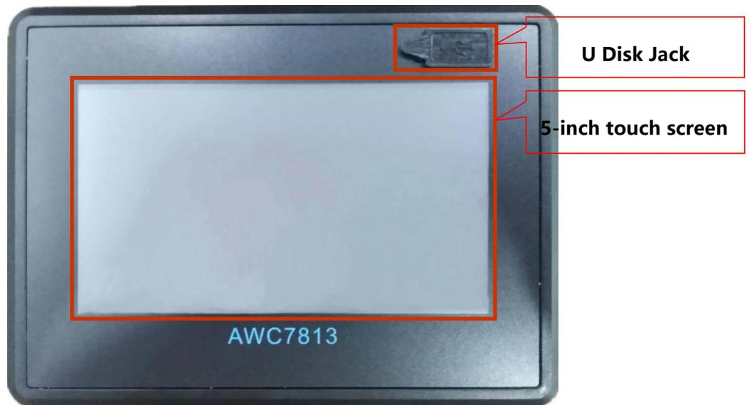
Figure1-5-2 Panel size diagram
