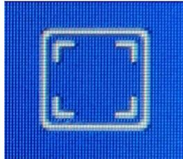
In the [Figure3-1-1 Main interface 1](#), click the **【 box 】** button, the laser head starts from the positioning point (the meaning of **【 Origin 】**, please refer to [3.2.7 Origin](#)), walking a rectangular around the outer frame of the graph at **【 RunBox'Speed 】** (For the definition of **【 RunBox'Speed 】**, please refer to [3.15.2.3 RunBox'Speed](#)), and it is a rectangular graph.
