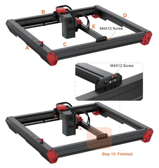
Step 16: Install a screw on E (X-Axis Assembly), tighten the screw until the belt is properly tightened (this means the laser module can move smoothly).
