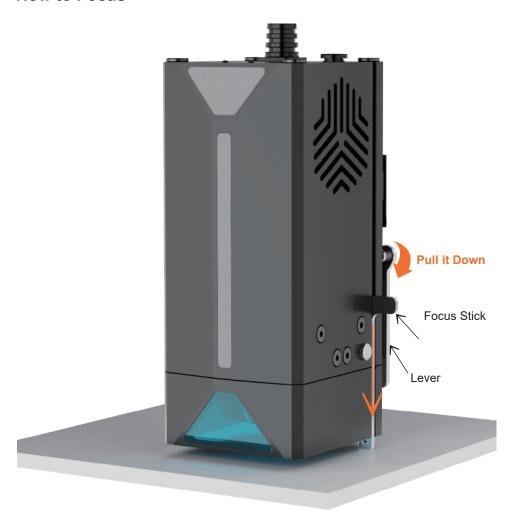
Step 20: Pull down the lever, let the laser module move down until the Focus Stick is against the engraved object,and then lift up the lever to fix the laser module.
