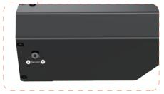
Step 17: Install two screws on D, tighten the screws until the belt of each side is properly tightened (this means the E (X-Axis Assembly) can move smoothly).
