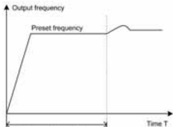
Figure 7-57 Sketch of closed-loop preset frequency operation
