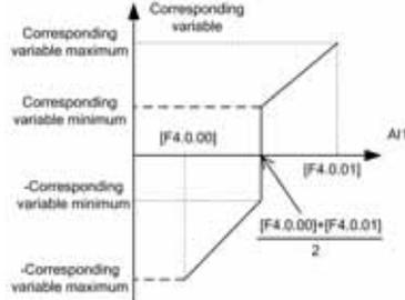
Figure 7-36-B Sketch of AI1 analog input and corresponding variables (bipolarity)
