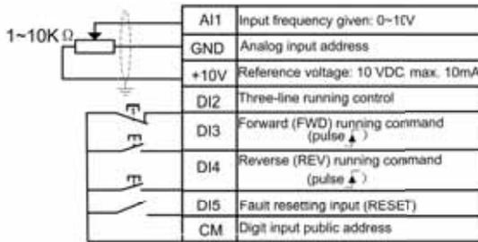
Figure 7-3 3 wire control 1/AI1 setting wiring diagram
