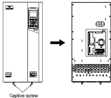
Figure 3-5 Schematic diagram of disassembly and installation of sheet-metal cover plate
