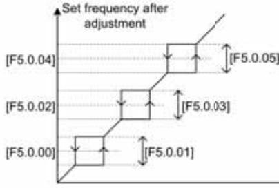
Figure 7-40 Schematic diagram of hopping frequency output
