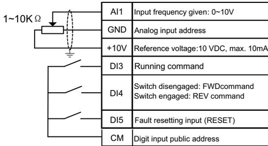
Figure 7-2-B 2 wire control 2/AI1 setting wiring diagram
