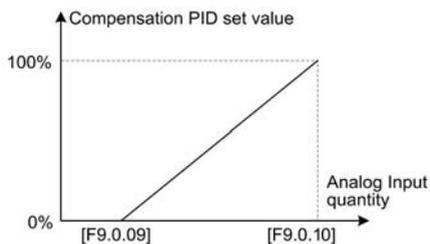
Figure 7-65 Sketch of compensation PID set value definition
