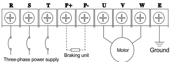
**Type X major loop terminal** Applicable type: V800-4T1600G/4T1850P ~ V800-4T3150G/4T3500P
