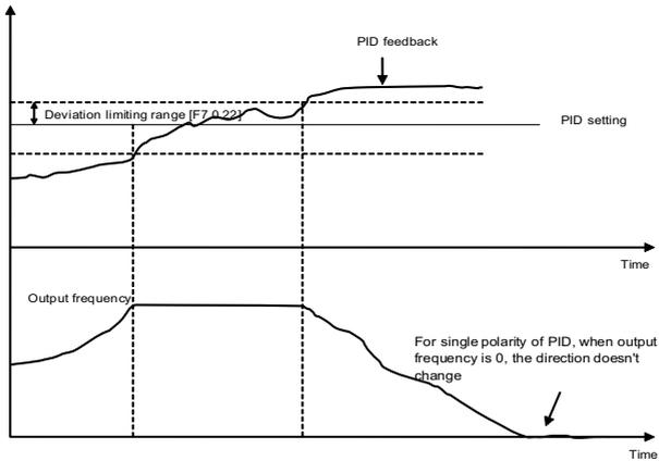
Figure 7-55-A Single polarity of PID control mode
