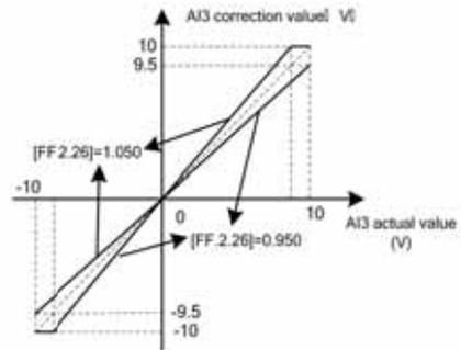
Figure 7-70-B AI3 gain correction curve
