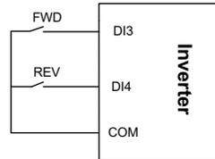
Figure 7-13-A Two wire running mode 1
