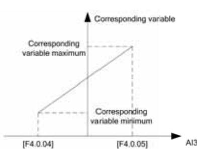
Figure 7-37-A Sketch of AI3 analog input and corresponding variables (unipolarity)
