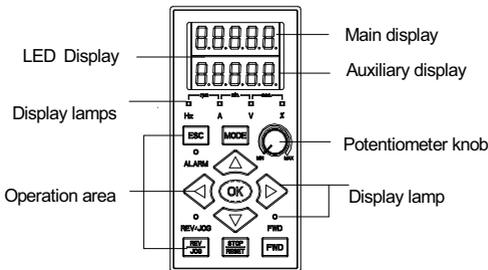
Figure 13-6-C double-line LED potentiometer panel
