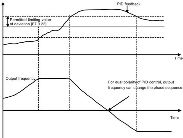
Figure 7-55-B Dual polarity of PID control mode
