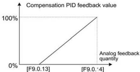
Figure 7-66 Sketch of compensation PID feedback value definition
