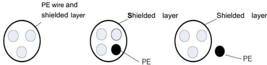
In order to restrain shooting and conducting of radio frequency effectively, shielded layer of shielded cable makes up of coaxial copper intertexture. For increasing shielding efficiency and conductive performance, intertexture density of shielded layer should be more than 90%.
