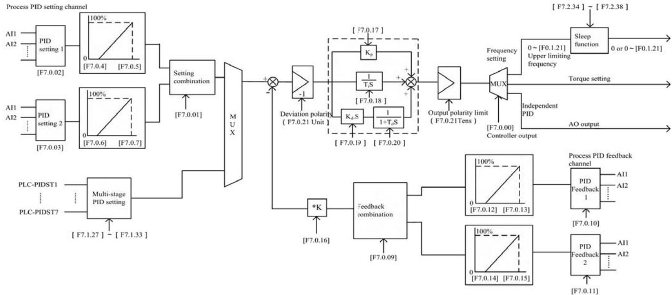
Figure 7-51 Schematic block of process PID control
