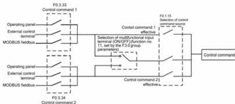
Figure 7-7 Sketch of selecting the control command sources
