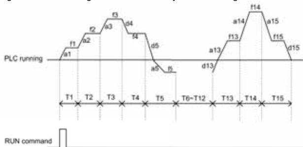
Figure 7-48-B Simple PLC operation single cycle mode
