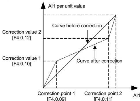
Figure 7-38 Curve correction of analog input AI1
