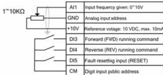
Figure 7-2-A 2 wire control 1/AI1 setting wiring diagram
