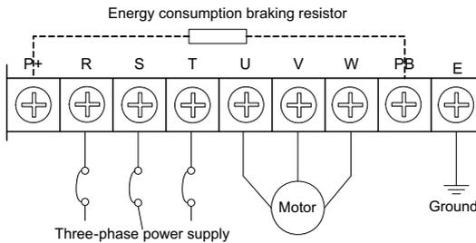
**Type III major loop terminal** Applicable type: V800-4T0075G/4T0090P ~ V800-4T0110G/4T0150P
