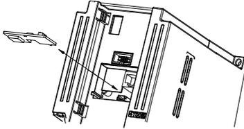
Figure 3-7-B installation and disassembly of type II function card
