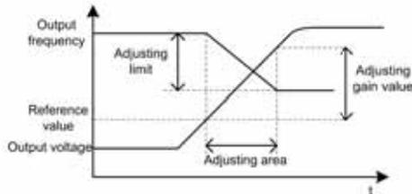
Figure 7-45 Sketch of load dynamic balance function
