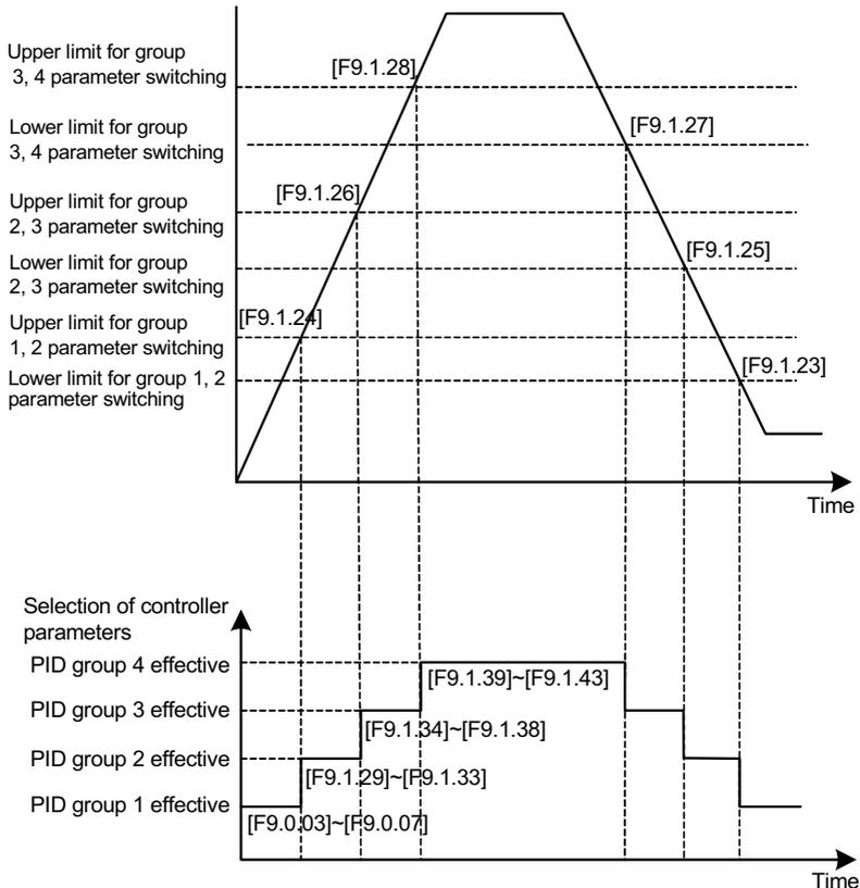
Figure 7-67 Sketch of compensation PID parameter switching
