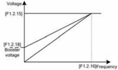
Figure 7-27-B Sketch of torque booster for constant torque curve
