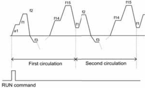
Figure 7-48-D Continuous cycling mode of simple PLC operation
