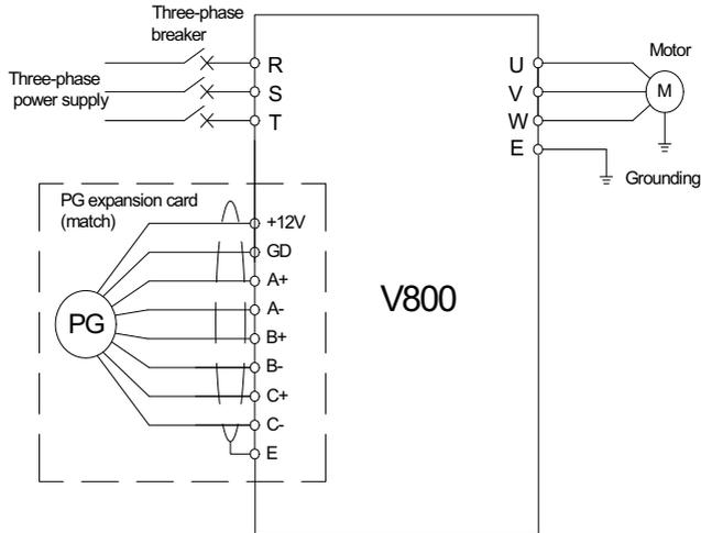
Figure 5-4 Wiring for the operation of VC mode
