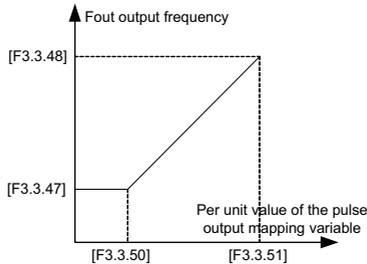
Figure 7-35 Characteristic curve of pulse output fount
