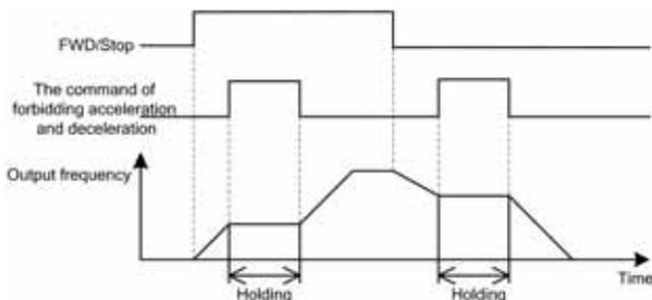
Figure 7-33 Sketch of acceleration and deceleration forbidden
