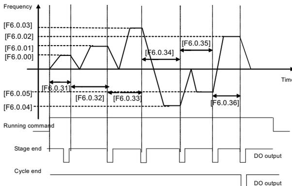
Figure 7-48-C Single cycle stop mode of simple PLC
